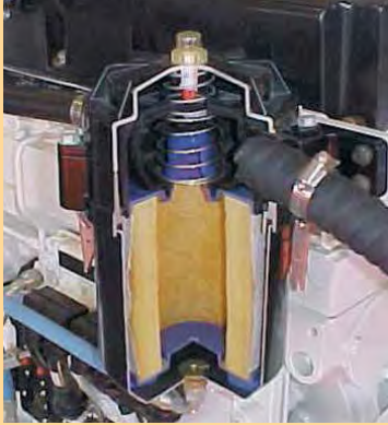
Cummins QSM11 marine engine with CCV cutaway
