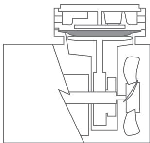
In reciprocating motion, with a short stroke, the diaphragm at the top of the connecting rod flexes up and down in a closed chamber, creating pressure or vacuum.
