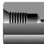
**M** - ANSI/ASME B1.20.1 external pipe threads
