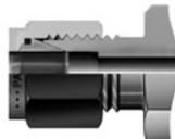
**F** - ANSI/ASME B1.20.1 internal pipe threads
