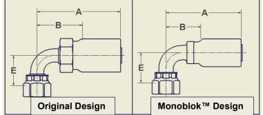
The introduction of these Parker 43 Series Monoblok fittings is a running change and will begin immediately. The new product will be packaged with a **bright yellow label containing the new cut-off factor**. For a short time, both designs will be in our inventory until the brazed version stock is depleted.
