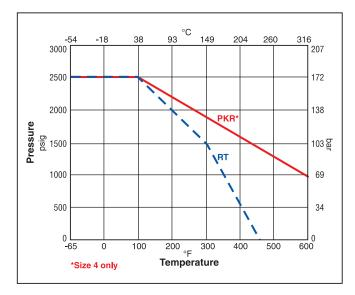
**Note:** This Pressure versus Temperature chart reflects the use of indicated seat materials in Stainless Steel valves without consideration of seal materials. When combining seat and seal materials, the most restrictive temperature rating of the seats or seals becomes the limiting factor on temperature range. Please refer to page 32 for seal temperature ranges.
