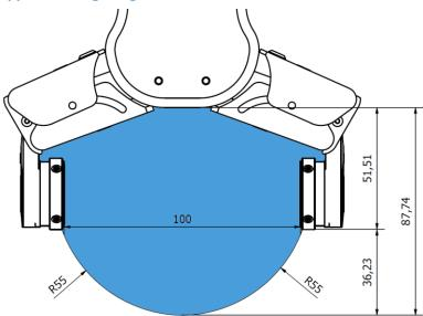
The dimensions are in millimeters.
