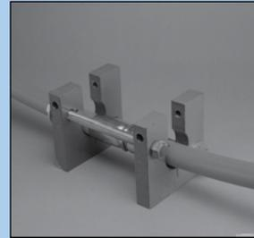
Place hose and fitting assembly into position on swager.
