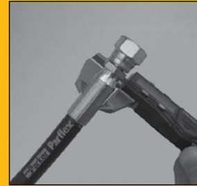
Measure crimp diameter of each fitting at top, middle and bottom of shell. Take measurements at a minimum of three places around shell circumference. Verify crimp diameter is within tolerances.
