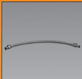
Slide two sockets over end of hose with bottom of sockets back to back. Position sockets at each end of hose.
