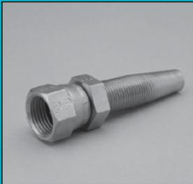
Inspect nipple for a through-hole, damaged or missing threads and improperly crimped nut (if applicable). Do not use if these conditions exist.
