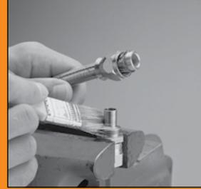
Using SAE 20 weight oil, lubricate nipple and socket threads. For stainless steel fittings use Parker ThreadMate™ or a molybdenum type lubricant.
