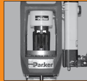
**Assemble hose** – Insert hose and fitting from bottom of crimper and up through die set. Position fitting so bottom of fitting skirt rests on the step (PARKALIGN® feature).
