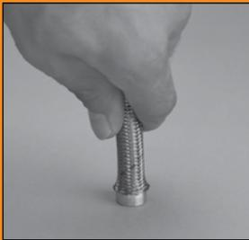
To complete positioning of sleeve, push hose end with sleeve against a solid flat surface.
