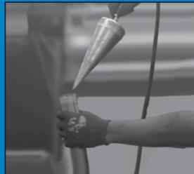
Blow ends of hose off / out to remove any debris left from cutting operation. Cut off wires or fabric extending past the end of hose.
