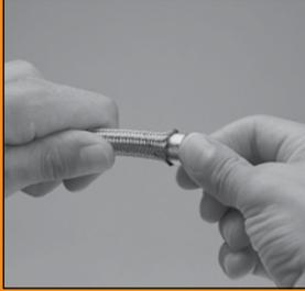
By hand, push sleeve over end of PTFE core tube and under wire braid.
