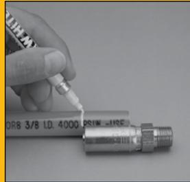
**Insertion Depth** – Shown is a 55 series fitting. See Hose Fitting Insertion Values, pg. G-43 for insertion depths of fitting series that do not incorporate an insertion depth. Mark hose end with proper insertion depth line.
