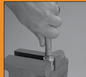
Push hose bore onto nipple to size tube and to aid in separating braid before assembling ferrule onto hose.
