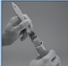
**Lubricate** – Using an SAE 20 weight oil, lightly lubricate inside of both hose ends.
