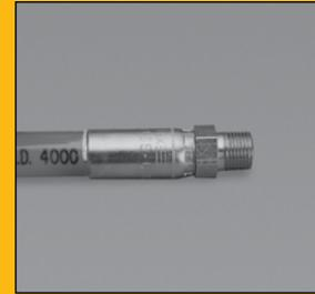
**Assemble hose** – Push hose into fitting all the way to depth insertion mark. (If fitting does not readily slide onto hose, perform the next step.)
