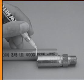
**Insertion Depth** – Mark hose end with proper insertion depth line. See Hose Fitting Insertion Values, pg. G-43 for insertion depths of fitting series that do not incorporate an insertion depth.
