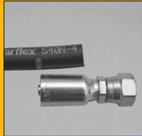
**Insertion Depth** – Shown is a 56 series fitting. Using Parflex Depth Insertion Block (part# TH9-1-56), mark the hose with the proper insertion depth line. On some fittings such as 55 Series, this depth is represented by a dashed or knurled line on the crimp shell.
