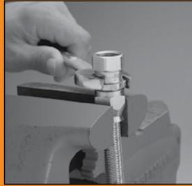
Wrench tighten nipple hex until clearance between hex and socket hex is 1/32" or less.
