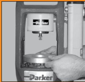
**Die Ring** – Place applicable die ring on top of die. Position ring so it is centered on die.
