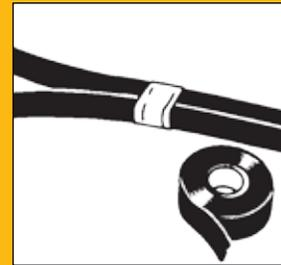
**Apply Tape** – At the option of the assembler, as dictated by the installation, a nylon lashing strap or tape may be applied at the termination of the separated length to provide protection against tearing of the web or hose covers.
