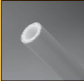
**Hose** – Visually inspect both ends of hose for square cut. Remove any burrs, loose fibers or wires.
