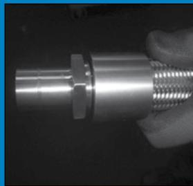
d. Pull collar out towards end of insert until at correct crimp position on insert of collar.
