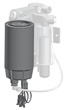
The RK12963 is a one-time retrofit kit for 90S1230C Integrated assemblies which incorporates a high quality water probe (with connectors), an indestructible metal bowl and a high-capacity 30 micron element. Once the retrofit from a 200200 element is complete, customers would then purchase the S3230P replacement element for their next service.
