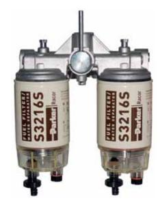
The Racor Dual Spin-On Series provides twice the filtering capacity in one compact and robust package. A shut-off valve located in the mounting head can switch to the clean filter so that the dirty filter may be serviced (servicing filters is not possible while engine is running).
