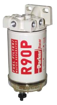
All 600 Series Spin-On fuel filter/water separators feature multiple fuel ports (4 inlets and 3 outlets) and a unitized mounting bracket for installation convenience. Inlet and outlet threads are 3/8"-18 NPTF for all models. These filter assemblies provide flexibility during mounting and fit any engine application.
