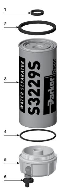
The standard B32029 bowl has no water sensor port. Bowls with water sensor ports are available as replacement kits (see item #5 above).
