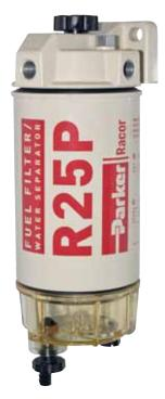
All 200 Series filters feature Spin-On, high-capacity, Aquabloc®II replaceable filter elements which separate water, remove solid contamination, and are available in 2, 10, and 30 micron.
