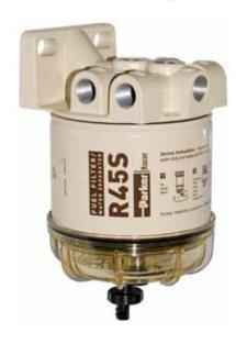
All 600 Series Spin-On fuel filter/water separators feature multiple fuel ports (4 inlets and 3 outlets) and a unitized mounting bracket for installation convenience. Inlet and outlet threads are 3/8"-18 NPTF for all models. These filter assemblies provide flexibility during mounting and fit any engine application.
