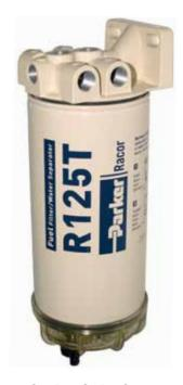
All 600 Series Spin-On fuel filter/water separators feature multiple fuel ports (4 inlets and 3 outlets) and a unitized mounting bracket for installation convenience. Inlet and outlet threads are 3/8"-18 NPTF for all models. These filter assemblies provide flexibility during mounting and fit any engine application.
