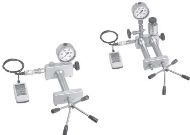
Typical test assembly „hydraulic“
