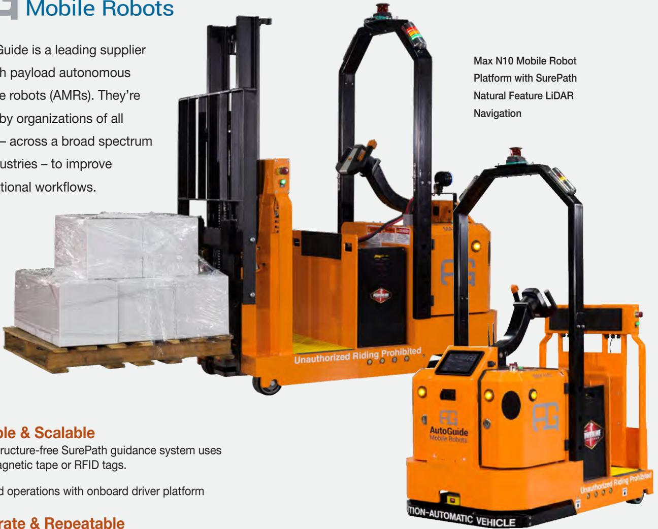
Max N10 Mobile Robot Platform with SurePath Natural Feature LiDAR Navigation
