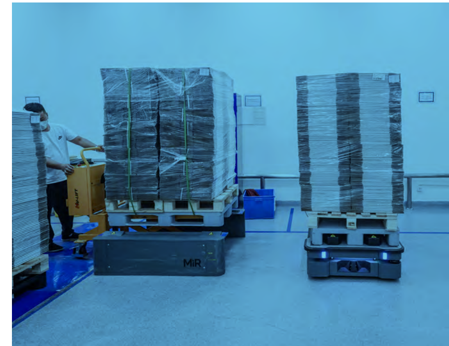
Novo Nordisk uses MiR500 robots equipped with MiR Lifts to automate the pallet transportation from docking bay to warehouse.
