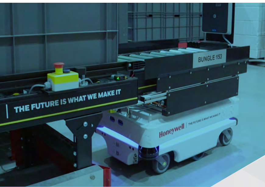
Honeywell has developed and integrated its own conveyor top module and an RFID scanner, so the MiR robots can scan the content of boxes and deliver them to the right production lines.
