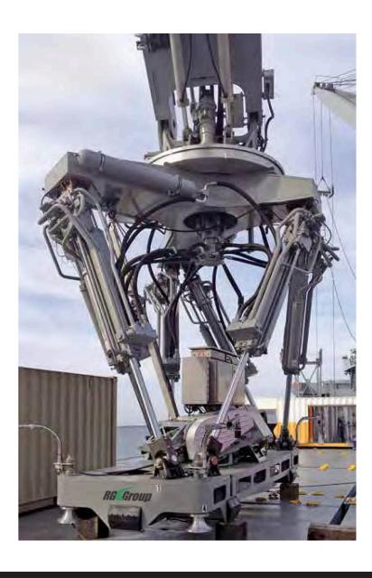
to ship at sea. This 1000 HP Hydraulic System moved the container at the end of the crane up to 7 feet vertically and in any multiple axis to keep the container aligned with the deck of the ship during all phases of ship-to-ship transfer up to and including Sea State 4. This RG solution exceeded all government requirements on budget and ahead of schedule.
