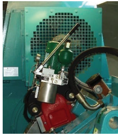
2. A diaphragm actuator is shown here of the manual brake actuator handle. The diaphragm accumulator stores a supplemental source of hydraulic fluid under pressure, which is used to actuate the caliper disk brake (shown in red) in the event of an overspeed of the rotor during a power outage. The silver “can” beneath the accumulator is part of the high-speed shaft hydraulic system. The gearbox is in the foreground, and the generator is in the background.
